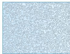
Vidrio templado Thermally Toughened glass
