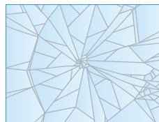
Vidrio Laminado Laminated Glass TRIPLEX glass with PVB membrane
